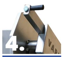
The push button on the handle supplies the machine with water and electricity (V401S).
